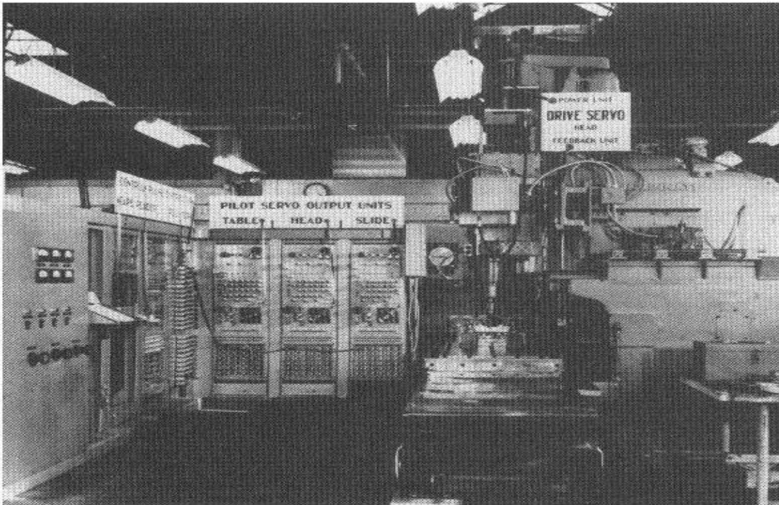
FIG.1.2.2 (a) The first NC machine, a retrofitted milling machine.
