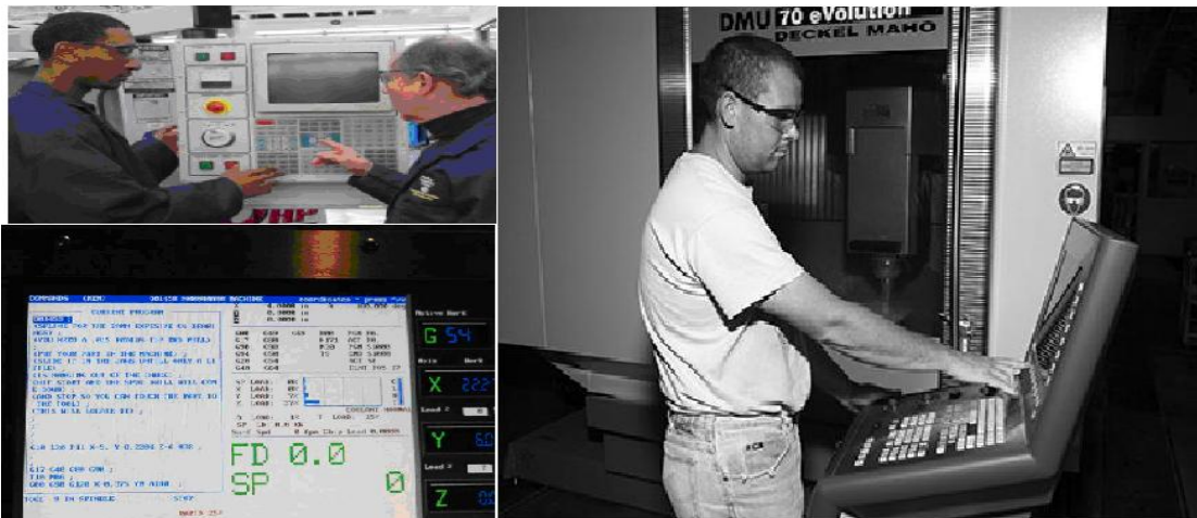
Fig.1.3.1 (a) Operators can introduce program data through the MDI in CNC manufacturing.
