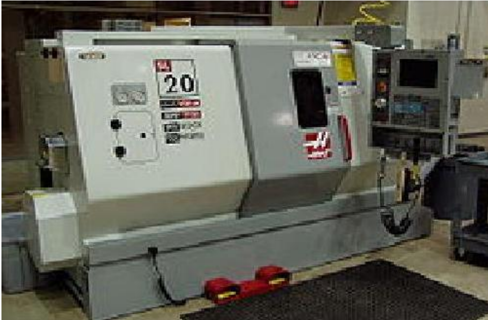
(Fig.1.3.1 a) Modern turning centre, see the MDI on the right side.
