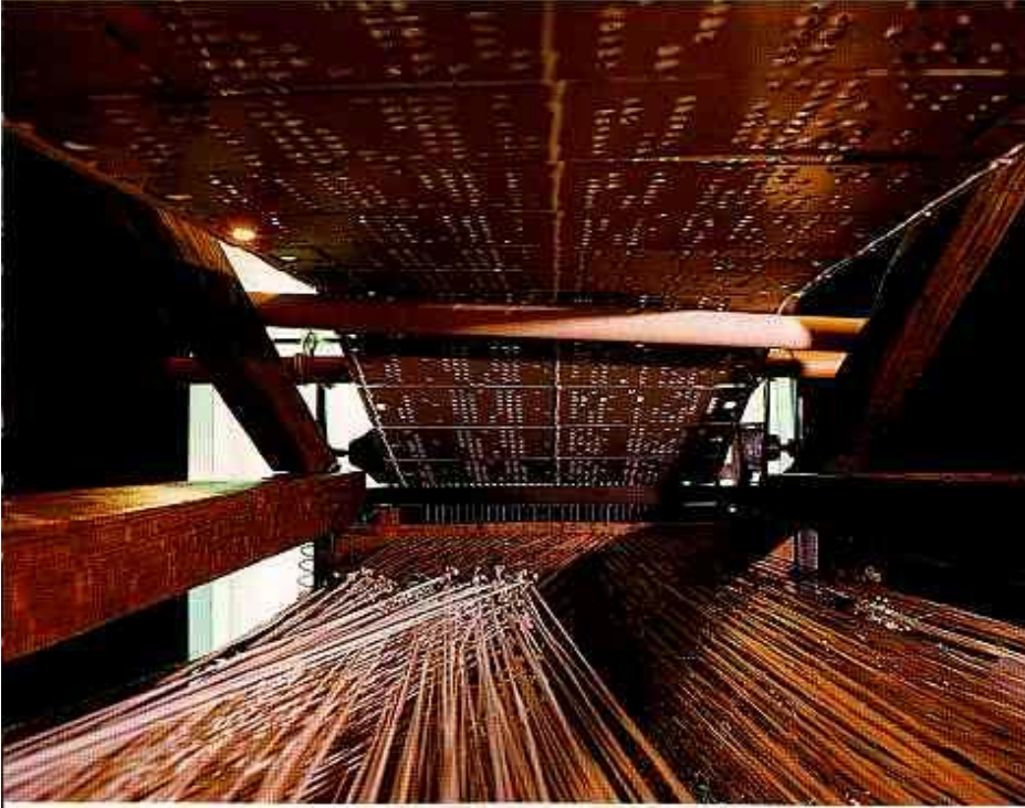
Fig.1.2.1 (a) Jacquard's Loom showing the threads and the punched cards
