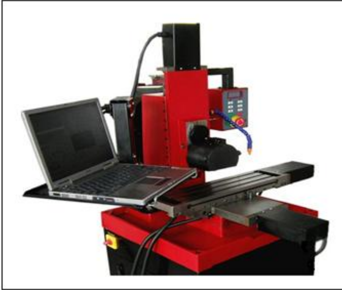
Fig.1.3.1 A CNC milling machine with a connection to a modern laptop.
