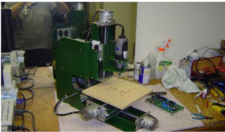
Fig.1.3.2.(b) A Carpenters CNC drilling machine.
