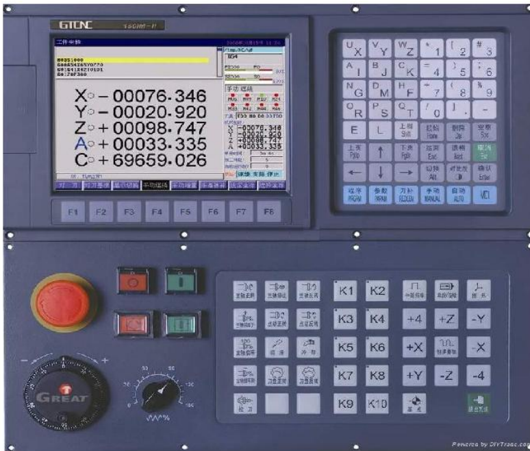
Fig.1.3.1 (b) MDI Control panel in modern CNC machines.
